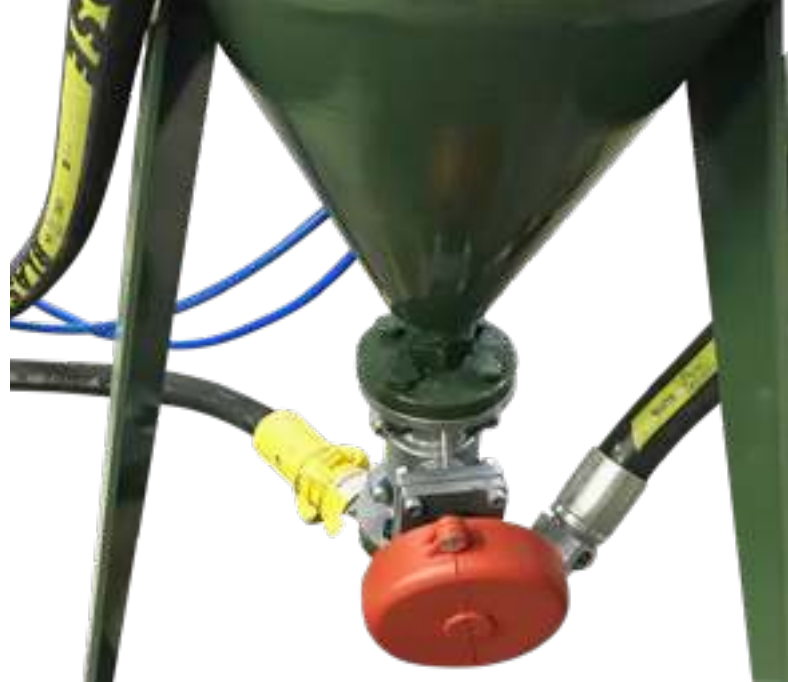
Anti-tamper guard (orange) fitted to a blast machine pressure regulator control
